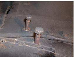
9. When installing the bracket and rack it may be necessary to grind slightly on the frame mount where the camber adjusters are for clearance. Some cars need this, others don't.
