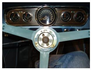
2. Remove steering wheel center nut and remove steering wheel assembly. Note a puller may be required to remove wheel.
