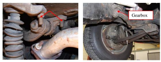
8. Remove the stock round crossmember from the vehicle and install the rack and pinion assembly in its place. Use the supplied bolts to put it in place and tighten to 65 ft.lbs.
