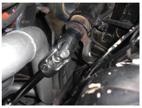
16. Verify that your rack is centered and set your toe adjustment by eye trying to keep the front wheels straight. Once you have this done install your steering wheel in place and tighten to 30 lbs ft. Reinstall the horn pad and take the car to a professional for an alignment. Enjoy the drive.
