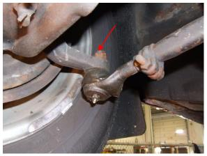
6. Remove the idler arm assembly and disconnect the pitman arm from the gearbox. Remove the entire steering linkage from the vehicle.
