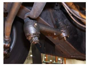
7. Remove the bolts that retain the gearbox to the frame and remove the gearbox by guiding it out of the vehicle and moving it toward the passenger side. Once the box and shaft assembly is out, set it aside, it will not be needed again.
