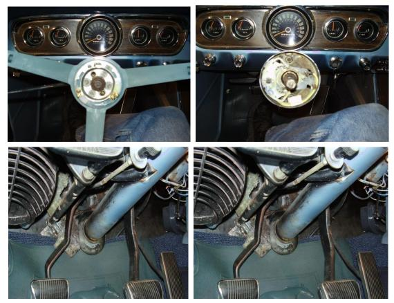
2. Remove the column tube assembly.
