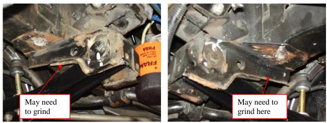
10. Once the bracket is installed you can now connect your outer tie rods to your steering arms. Note the kit has been shipped to you with 2 sets of tie rods. You need to determine which ones you use by comparing the taper size of your stock tie rod. Be sure that the tie rod you select fits your steering arm tightly and locks on the taper.
