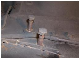
9. When installing the bracket and rack it may be necessary to grind slightly on the frame mount where the camber adjusters are for clearance. Some cars need this, others don't.
