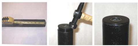
5. Once you have this done install the appropriate floor plate provided in your kit using the hardware provided. Slide the floor plate over the column tube with the clamp and install the column through the firewall and bolt back in place. Attach the new floor plate with supplied hardware and complete the installation.
