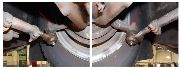
6. Remove the idler arm assembly and disconnect the pitman arm from the gearbox. Remove the entire steering linkage from the vehicle.
