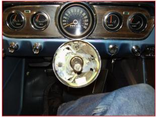
3. From under dash remove the bolts that retain the column tube to the dash. Remove the 3 screws at firewall where the column goes through and remove retainer plate.
