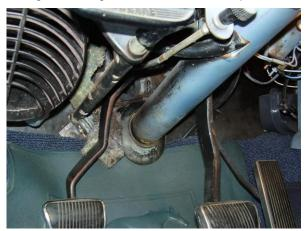
4. Remove the column tube assembly from the vehicle. Be sure to save the pinch bushing at the top of the steering shaft and column tube, you will need to reuse this piece.
