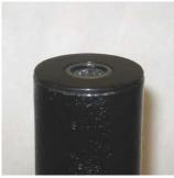
12. Install supplied brass washer and u-joint. With both of these pieces installed, make sure there is not a gap between the lip of the bushing and the end of the steering column.
