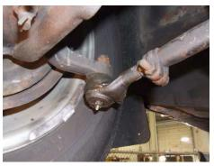
6. Remove the idler arm assembly and disconnect the pitman arm from the gearbox. Remove the entire steering linkage from the vehicle.
