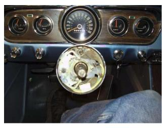
3. From under dash remove the bolts that retain the column tube to the dash. Remove the 4 screws at firewall where the column goes through and remove retainer plate.
