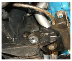
6. When you have replaced all four bolts with longer set, install four one-inch standoffs over bolts.
