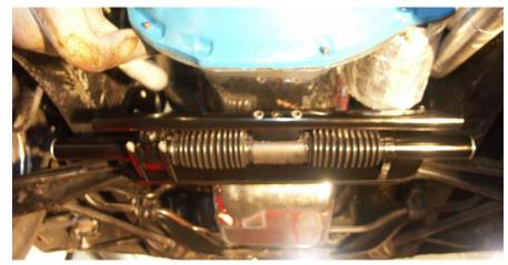
8. Install outer tie rod ends in knuckles and leave nuts loose. <u>NOTE:</u> Your kit has been shipped with 2 sets of outer tie rod ends. Please check the taper fit on your spindles and use the appropriate ends for your application.
