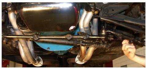
3. On passenger side, remove the three bolts on the idler arm assembly.
