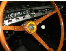
6. Remove nut that retains wheel and remove the wheel. Note: It may be necessary to use a puller to remove wheel. Do Not Pry Off! You may crack the wheel.
