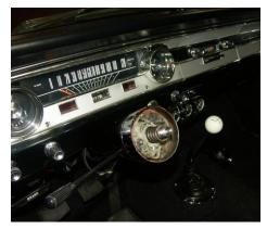
7. When wheel is removed go under the dash and disconnect wire harness from column to vehicle. **Note:** If vehicle does not have a hard-shell connector, disconnect one wire at a time and mark with number stickers.
