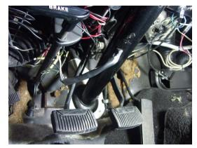
8. Remove two retaining bolts under dash that secure column to dash and remove steering column shell. **Note:** Do not lose ring around shaft.
