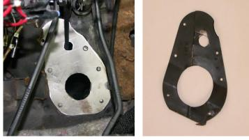
4. Install column tube and hardware (leave loose). **Note:** Do Not Install Shaft Yet. From under car, install column clamp over tabs on column plate and leave loose.
