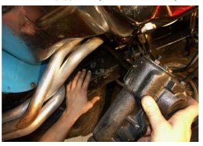
10. From under dash, remove six sheet metal bolts that retain to column support place to firewall and floor. Remove plate and discard.
