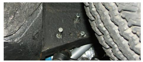
4. On driver side, remove attaching nut from linkage to gearbox & remove complete steering linkage from vehicle.
