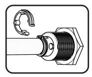
STEP THREE REMOVE PLASTIC CLIP BY PUSHING ON TABS. DISCARD CLIP.
