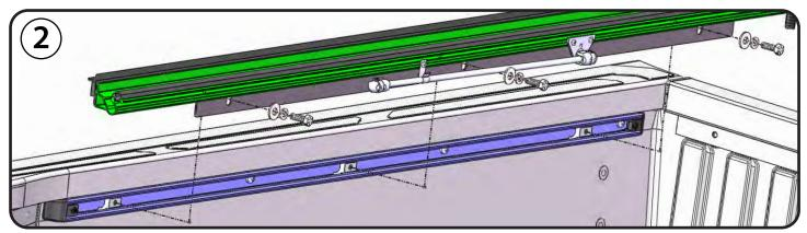
Slide the clamp assembly (3 per side) into the Utility rail, position one front, one center and one rear, Figure 1.
