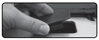
After the install is complete, snap the stake pocket covers into the stake pocket holes.
