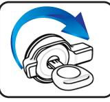
STEP TWO ROTATE CLOCKWISE 180 DEGREES
