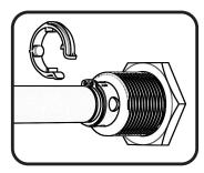
IF KEY IS NOT FULLY INSERTED PRIOR TO ROTATING - DAMAGE TO LOCK WILL OCCUR.
