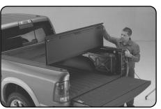
2 If this is as far as you would like to open the cover, you can secure it in this position. Release the strap from the stowed position by squeezing the tabs. Attach the buckle at the bulkhead, pull the strap to take up the slack and secure the cover.
