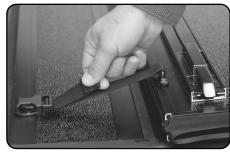
Pull the cable on the last panel and fold the cover up towards the cab.
