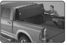
4 Secure the cover by attaching the prop rods. Remove the prop rod from the j-clip on the cover mounting rail. Attach to the cover by pressing onto the ball stud. To close simply reverse this process.
