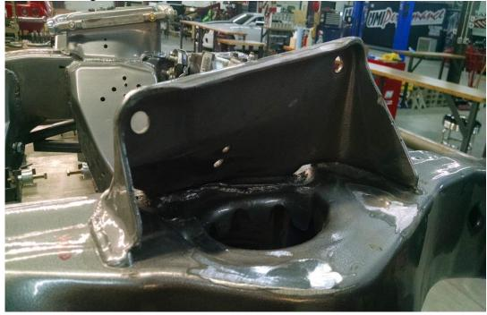
5. Lay the supplied template flat in the area to layout the portion to be cut for coilover clearance. It is recommended to cut short and grind to fit. Use the supplied ring to test fit. When satisfied with fitment, tack weld the ring in place, it is not recommended to fully weld at this point.
