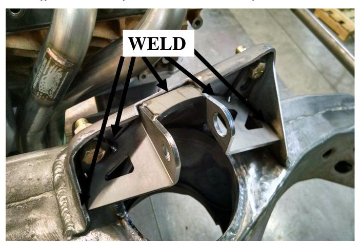
10. Weld the factory seams of the upper a arm mount as shown below. This helps reinforce the factory mount.
