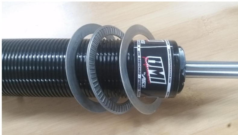
Figure 4 – Assembling Thrust Bearings on Shock
