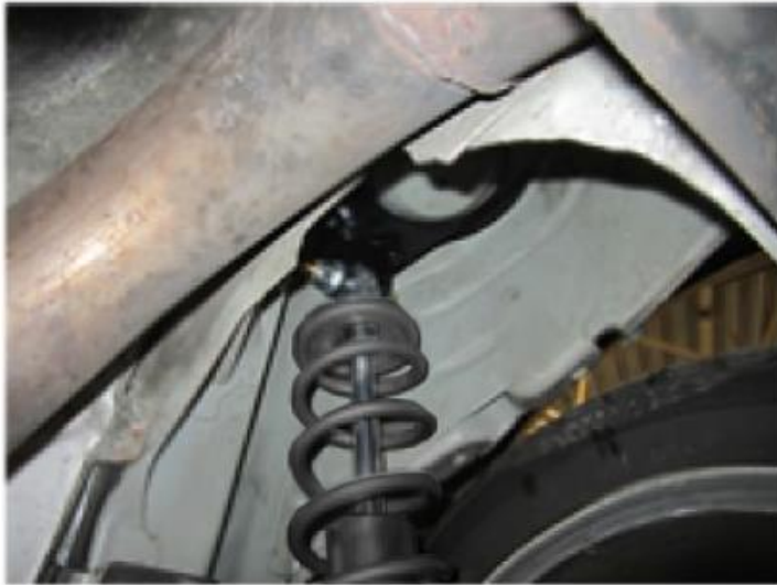
Figure 7 – Upper Bracket Installed
