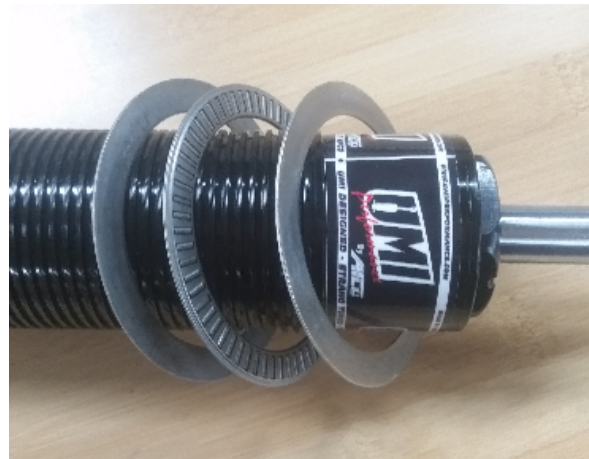
Fig 2 – Assembly order (optional bearing and washer)
