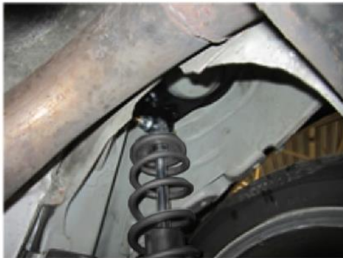
Figure 7 – Upper Bracket Installed Note: Shock may be installed spring up or spring down however UMI recommends rod and adjuster down for easy adjustment.
