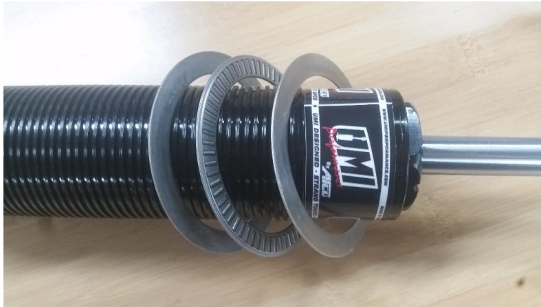
Figure 4 – Assembling Thrust Bearings on Shock
