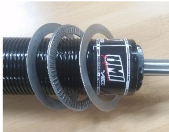
Fig 2 – Assembly order (optional bearing and washer)
