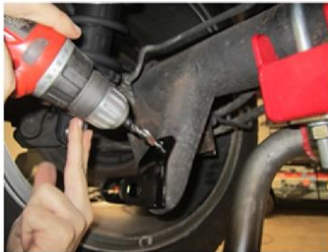
Figure 3 – Drilling for 3/8" Reinforcement
