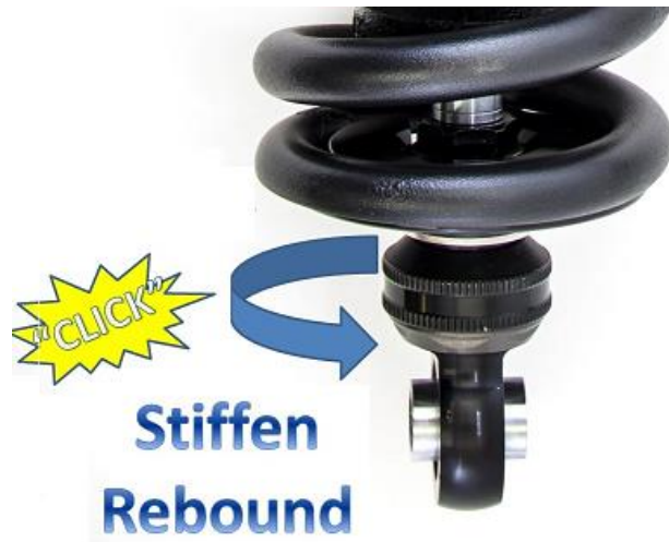
Figure 5 – Start rebound adjustment on 20 clicks (from full stiff). UMI suggests making adjustments 2 clicks at a time.
