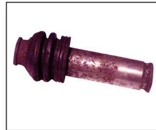
Sliding pins and bushings must be lubed with the proper lube if they are to operate properly.
