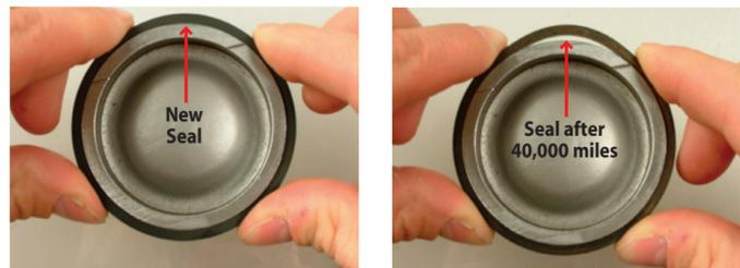
Heat and time dry out the **square-cut seal** and reduce the amount of pull-back as the seal ages. A new seal will pull back the piston about 0.015 inch. In comparison, an old seal may only pull back 0.010 inch or less. If the piston does not retract, it can cause the pads to drag, wearing the pads prematurely.
