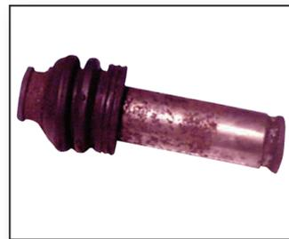
No lubrication on bushings and/or pins prevents free movement.
