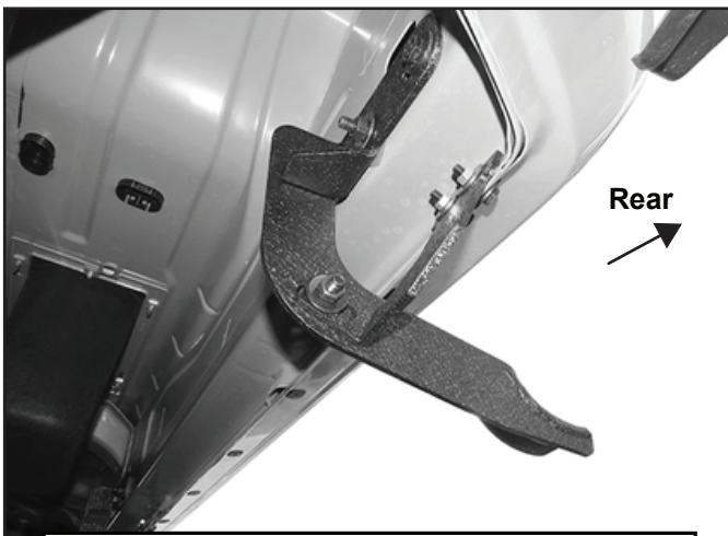
(Fig 17) Passenger/right rear Brackets installed
