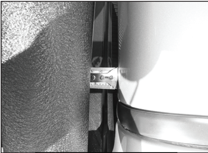
(Fig 9) Front Cross Tube must be at least 30mm from the rear of the cab
