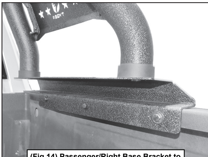
(Fig 14) Passenger/Right Base Bracket to bed installed
