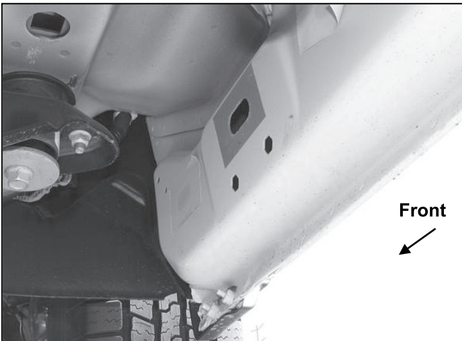
(Fig 1) 2009-mid 2015 Passenger front mounting location (No factory holes in pinch weld 2009-2012 models)
