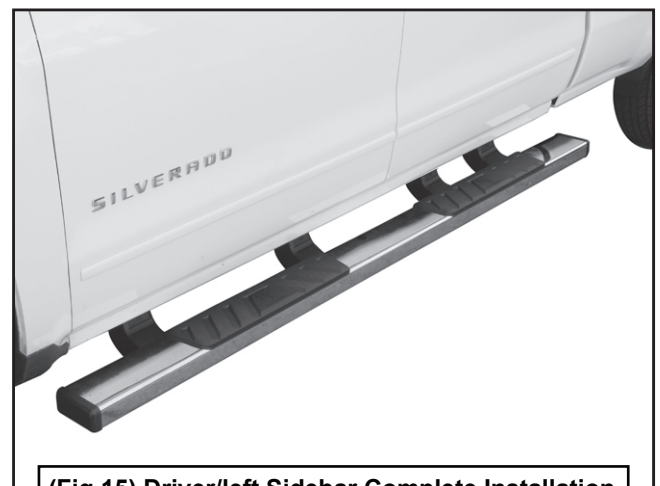
(Fig 15) Driver/left Sidebar Complete Installation
