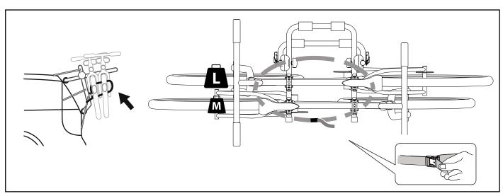
GB-US - Double check that all the straps are correctly tightened after installing the bikes
