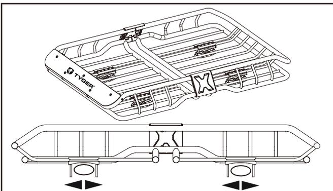
**Step 7:** Install the basket on the crossbars. The distance between bars should not be less than 21" or more than 30". Slide the kits to fit on the bars. Make sure the basket is centered.
