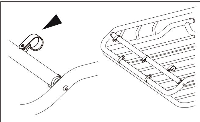
**Step 3:** Insert the 5 plastic clamps on the front tube. Position 3 at the top and 2 at the bottom as illustrated here.
