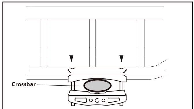
**Step 8:** Insert the lower clamp of the attachment kit under the crossbars. Matching the clamp above and under the crossbar. Balance the tightening force one screw to the other. Tighten firmly.
