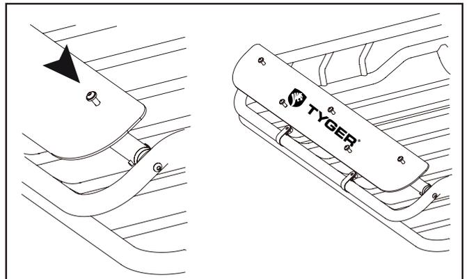
**Step 4:** Use 5 screws M6x16 to attach the deflector to the basket front part using the 5 clamps installed in step 3.
