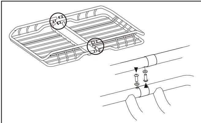
**Step 1:** Assemble front basket to rear basket using 4 screws M6x16 and 4 washers. Firmly tighten all the screws.
