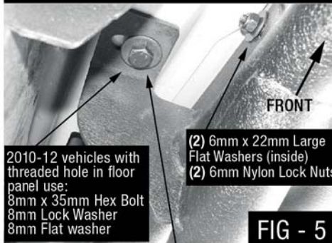
07 - 10 with "open" floor panel using 10mm Nut Plate: 10mm x 35mm Hex Bolt, 10mm Lock Washer, 10mm Flat Washer
