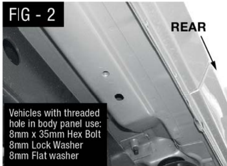
Example of 2010-12 "closed" floor panel with threaded hole-Nut Plate not required
