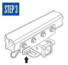
Insert the trailer wiring, if equipped, into the trailer wiring mounting tab on the receiver as shown. Installation is now complete.
