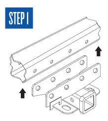
Slide the receiver over the rear crossmember, taking care to align the 4 holes in the receiver with the 4 holes in the cross member. Once in place, insert left or right most bolt with flat washer into the back side of the hitch and throught the cross member. Place the nylock nut and flat washer on to the bolt. Secure but do not tighten.
