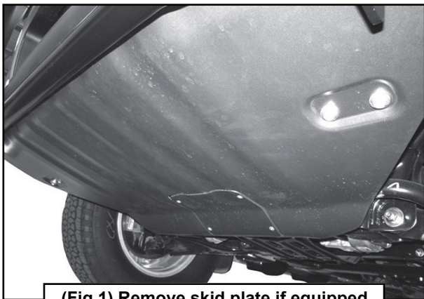
(Fig 1) Remove skid plate if equipped
