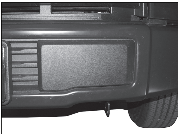
(Fig 5) Remove bumper pads to access splash guard hardware if necessary. 2015 F150 pictured
