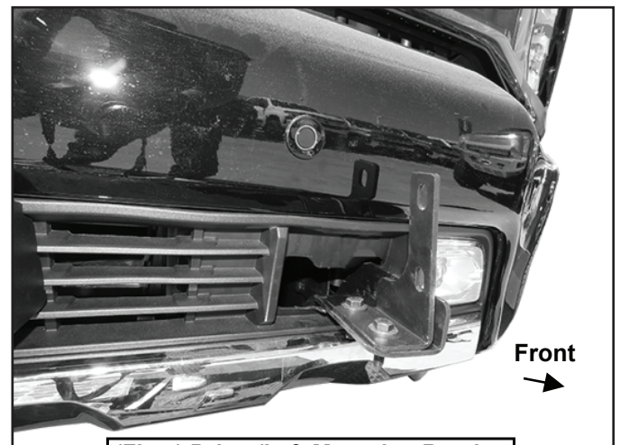
(Fig 7) Driver/Left Mounting Bracket attached to the Frame Bracket
