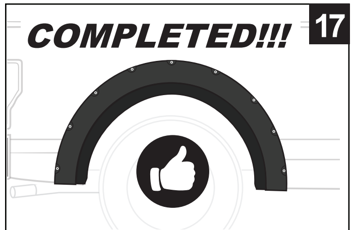
17. Tighten all 5 screws from STEPS 14-15 to complete installation. Repeat STEPS 8-17 to the other side.
