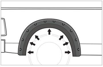
**STEP 13:** Apply pressure on flare and tighten all screws. Installaion complete.
