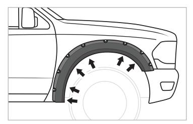
$\ensuremath{\mathbf{STEP}}$  5: Apply pressure on flare and tighten all screws. Installaion complete.
