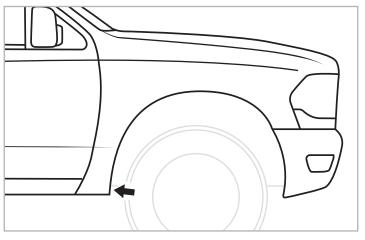
**STEP 1:** Start from rearward mudflap on the front passenger wheel well.
