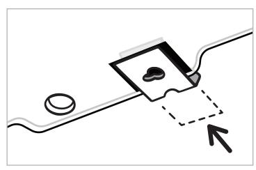
**STEP 9:** Stick a supplied Tab **[F]** over the factory hole and slide a supplied U-clip **[G]** over the Tab as shown.
