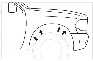
**STEP 3:** Remove 4 factory screws from the wheel well for the shown positions with 8mm socket. Screws will be reused in STEP 4.
