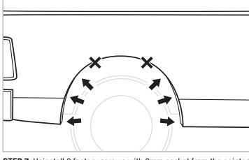
**STEP 7:** Uninstall 6 factory screws with 8mm socket from the pointed positions. (Keep the X location screws installed) Hold onto screws to be reinstalled in STEP 12.
