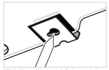
STEP 10: With an awl, poke a hole in the Tab through the U-clip.
