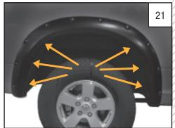
Hold flare in place start six supplied screws by using an Phillips Head Screwdriver. Do not tighten.
