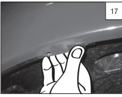
Install plastic tab over existing factory hole. There is two holes and it's the one on the right.
