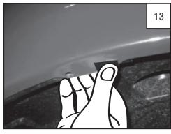
Install Tab over existing factory hole as shown in STEP 14.
