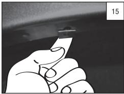
Install U-Clip over Tab installed in STEP 13.
