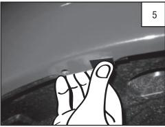
Install Tabs over factory hole locations shown in STEP 6. For location 2, install the tab over the factory hole located more towards the front of the vehicle.
