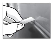
Using the Edge Trim Tool to seat edge trim against vehicle by hooking curved end under edge trim at one end of flare. Next, slide around outer edge of flare to the other end.
