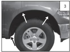
Start with passenger side. Using an 8mm socket wrench, remove 3 factory screws.
