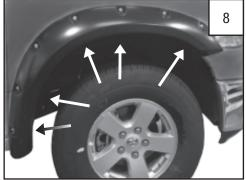
Hold flare in position. Using a Phillips screwdriver, install 5 supplied PH Screws. Do not tighten.
