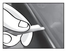
Using flat end of Edge Trim Tool, seat edge trim against flare by inserting straight end between edge trim and flare at one end. Next, slide around entire edge to the other end.
