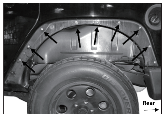
(Fig 16) 6mm Threaded Inserts installed
