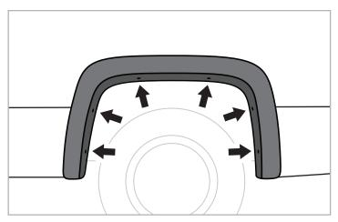
**STEP 4:** Position rear flare in place by aligning up holes in flare with vehicle's existing factory holes.
