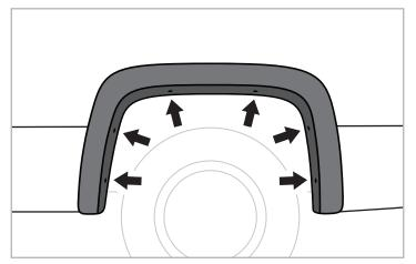
**STEP 5:** Starting at the top center, install 6 supplied Tufloks.
