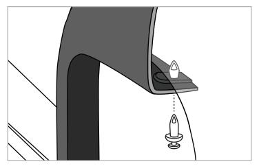
**STEP 3:** Insert the supplied Tuflok **[A]** through holes in flare and into vehicle's factory holes.
