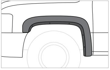
**STEP 1:** Position front flare in place by aligning up holes in flare with vehicle's existing factory holes.
