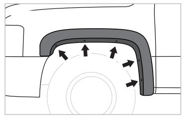
**STEP 2:** Starting at the top center, install 6 supplied Tufloks.
