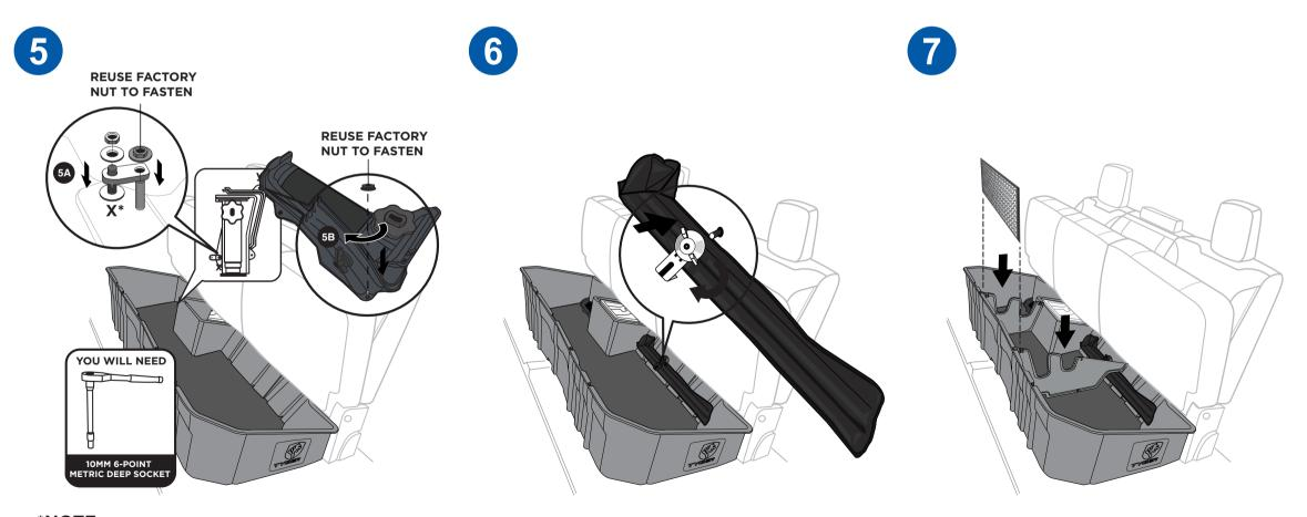
\*NOTE: APPLY PROVIDED HARDWARE KIT THROUGH HOLE (X) TO FASTEN THE JACK
