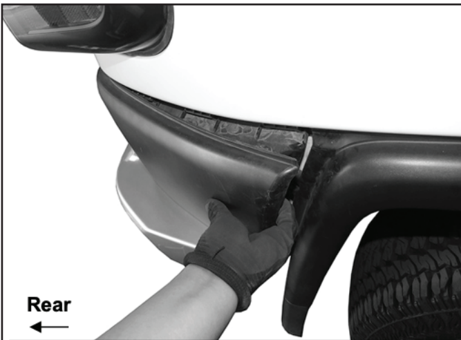
(Fig 5) Pull end of bumper cover outward to release from clips (passenger/right side pictured)
