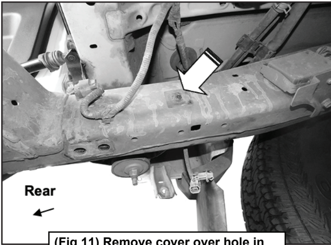
(Fig 11) Remove cover over hole in frame (arrow-driver/left side pictured)
