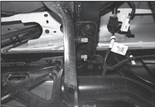
(Fig 1) Unplug and remove 7-wire trailer plug, unplug license plate lights and sensors if equipped
