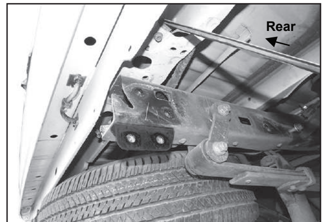
(Fig 8) Passenger/Right Frame Mounting Location with the Support Bracket attached (Models without hitch)
