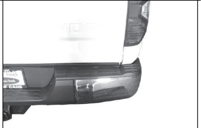
(Fig 2) Use a flat blade screwdriver to pry the plastic cover from the top of edges of the bumper
