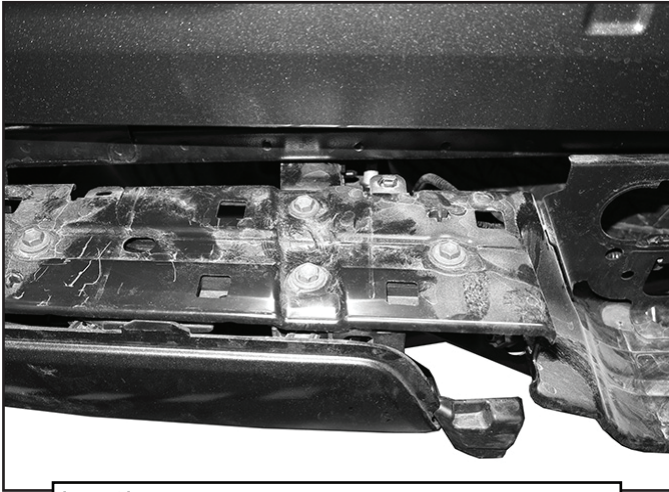
(Fig 3) Models with receiver hitch, remove the hex bolts attaching bumper to top of hitch
