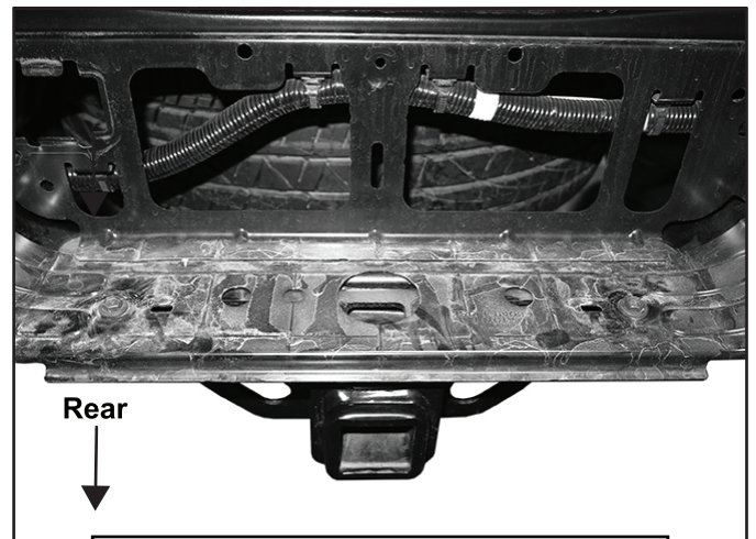
(Fig 2) Models with receiver hitch, remove plastic cover from top of bumper
