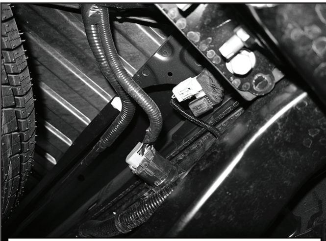
(Fig 1) Unplug and remove 7-wire trailer plug, unplug license plate lights and sensors if equipped
