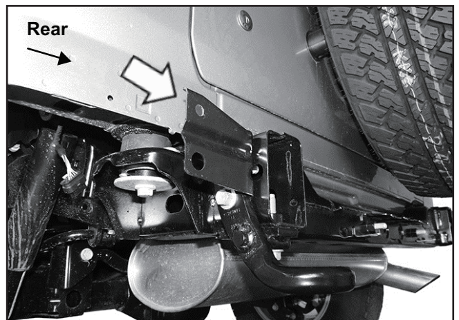
(Fig 5) Remove tow hook and inner bumper bracket from side of frame
