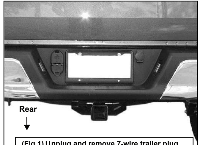
(Fig 1) Unplug and remove 7-wire trailer plug
