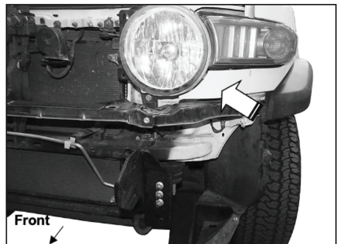
(Fig 14) Temporarily remove driver/left body fill panel below turn signal assembly (arrow)
