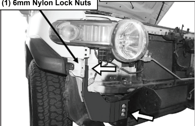
(Fig 16) Passenger/right installation of Lower Body Cover illustrated. Attach mounting tab on top of Cover to back of tab on body (arrows)
