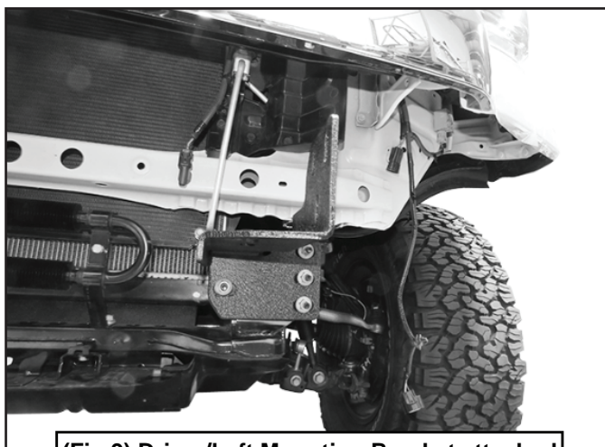
(Fig 9) Driver/Left Mounting Bracket attached
