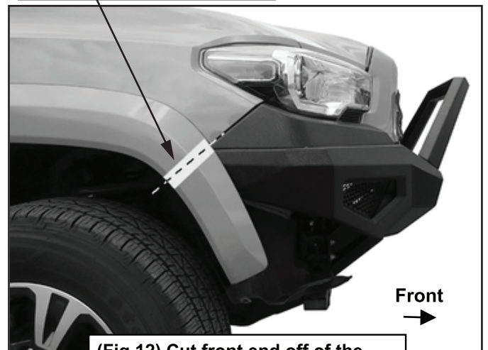
(Fig 12) Cut front end off of the fender flare to match up to Bumper
