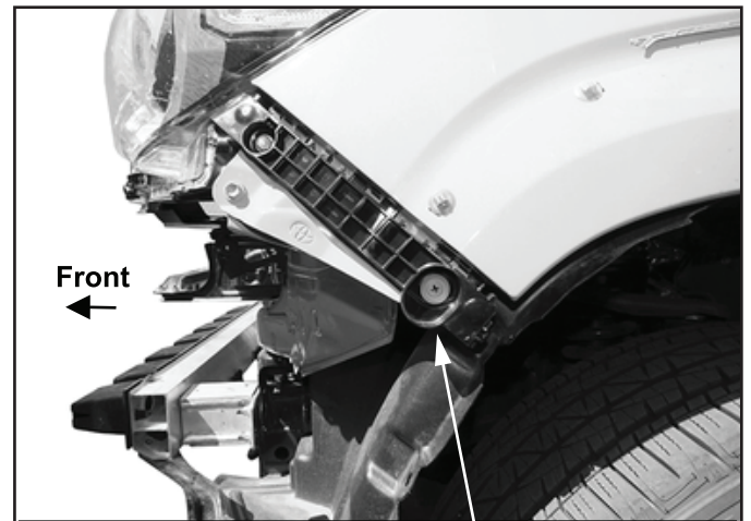
(Fig 3) Remove plastic block (arrow) from front edge of fender. Reinstall hardware to secure headlight
