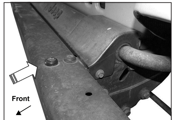
(Fig 2) Remove bumper bolts from top of bumper (arrow). On TJ-LJ models, also remove plastic sway bar cover from frame
