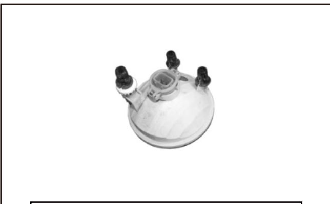
(Fig 12) Remove the fog light bulb from the plastic bracket assembly (see Fig 11)
