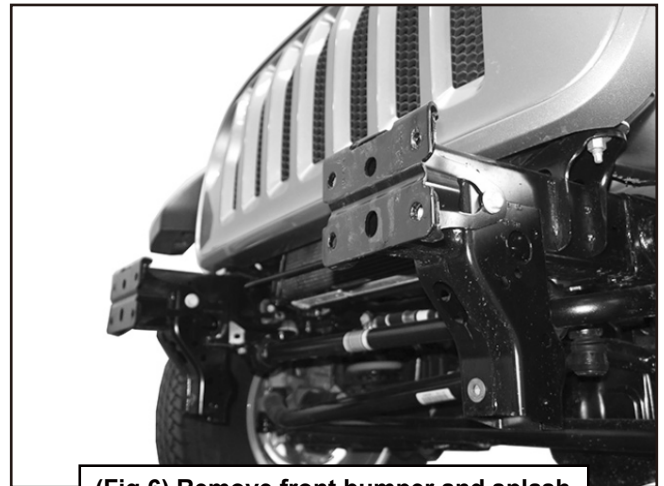
(Fig 6) Remove front bumper and splash guard or skid plate (2018-on JL pictured)
