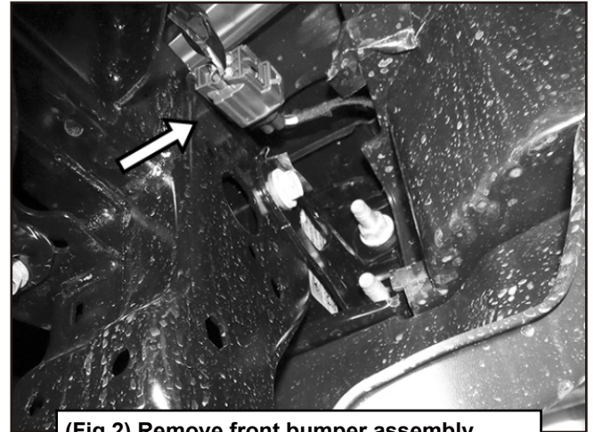
(Fig 2) Remove front bumper assembly (driver side JK outer bumper bolts pictured)
