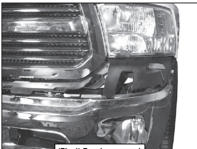
(Fig 4) Fascia removed
