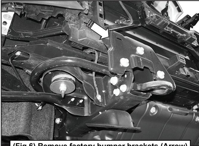
(Fig 6) Remove factory bumper brackets (Arrow)
