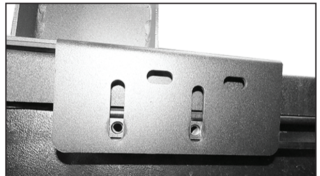
(Fig 14) With assistance, place the Overland Bed Rack assembly onto the top of the bed. Line up the Block Nuts to the desired slots, (2) Block Nuts per mounting plate
