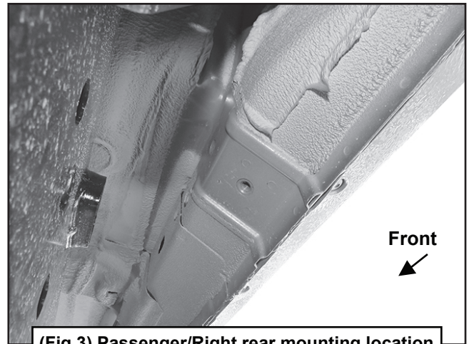
(Fig 3) Passenger/Right rear mounting location
