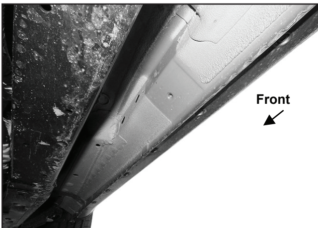
(Fig 2) Passenger/Right center mounting location
