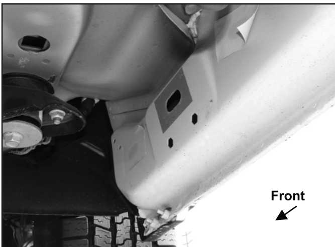
(Fig 1) 2009-mid 2015 Passenger/Right front mounting location (No factory holes in pinch weld 2009-2012 models)
