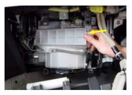
5. Unlatch the filter cover by pulling from the right side of cover. Replace with new TYC filter. Ensure the filter arrow is pointing up.
