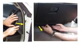
1. Remove the right side cover by pulling as shown in the picture and set it aside.
