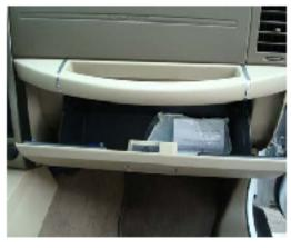
1. The filters are located behind the glove compartment. Remove the glove box by pulling the glove compartment downwards.
