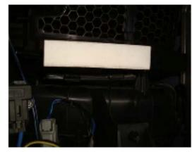
Slide out the old filters and install new TYC filters. (TYC filters come in a set of 2) Ensure that the Air Flow arrow is pointing down for both filters.
