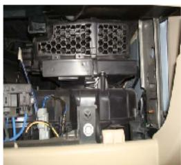
After the glove box is removed, the filter access door is visible. Pull on the locking tab on both sides remove the door, exposing the filters inside.
